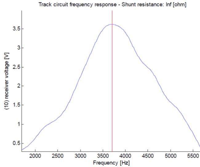
**Fig. 6.** Frequency response analysis of a track circuit
