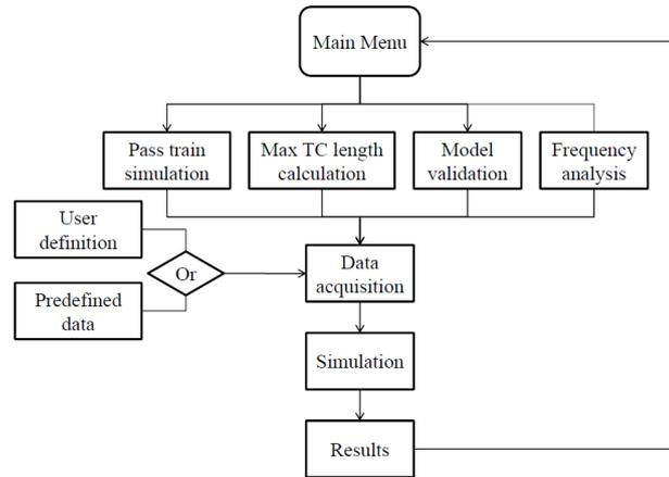
**Fig. 4.** Software blocks diagram
