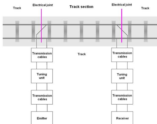
**Fig. 2.** Track circuit model
