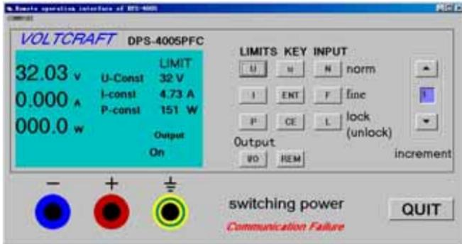
Indication on the PC is complete same as the distribution of front panel and LCD display on the power supply. Operating of the PC is same as the power supply, except that click the “L” key three times to release the operating elements (unlocked). In additional, it increases an increment window on the PC, and the step of up/down can be set in the window.
