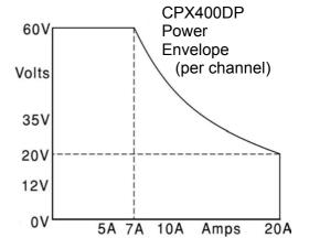
Operating Ranges: Four selectable ranges: 60V/20A, 60V/7A, 20V/20A and Custom Limits.
