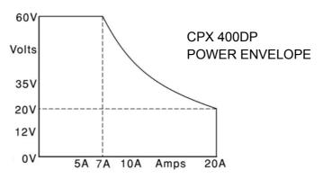
The power envelope is set to give 60V/7A, 42V/10A and 20V / 20A under all supply conditions (both outputs loaded); at lower output voltages the output power is restricted by the 20A current maximum.
