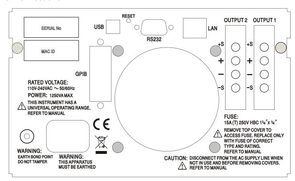
The output and sense terminals for OUTPUT1 and OUTPUT2 are duplicated on the rear panel terminal blocks and are marked +O/P, -O/P, +S and -S. These connections are paralleled with their front panel equivalents.
