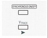
Pressing  $V_{TRACK}$  selects voltage tracking mode. The two outputs remain electrically isolated but the Voltage controls of Output 1 (the Master) set an identical voltage on Output 2 (the Slave).
