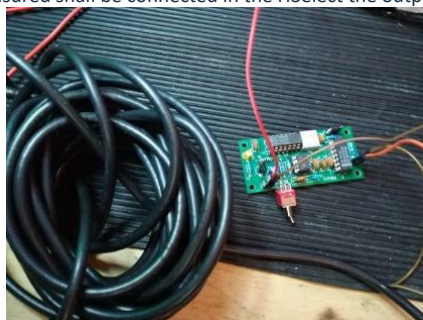
TDR Coaxial cable measure
