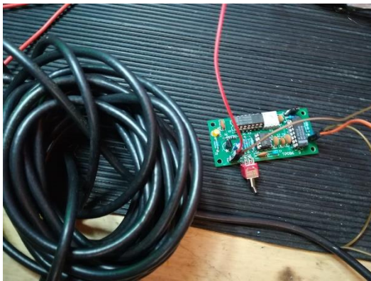
TDR Coaxial cable measure
