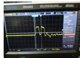
TDR Coaxial cable Pulse shape
