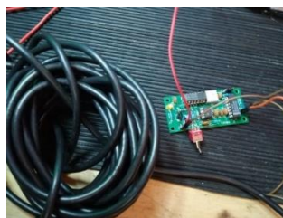
TDR scope time delay measurement
