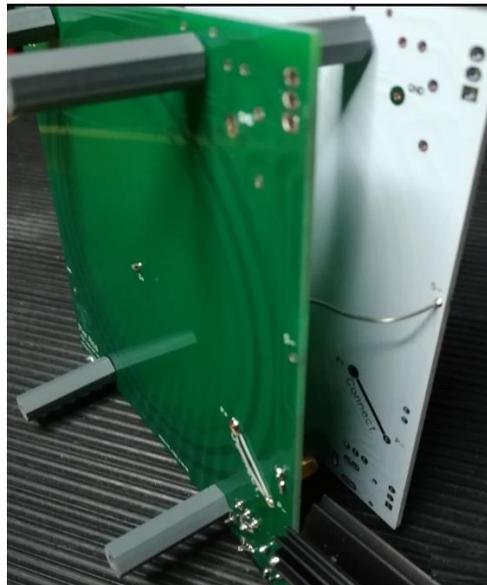
Connection of 2 PCB in series: a metallic joint shall be done between S+ reference of PCB 1 to S- reference of PCB2
