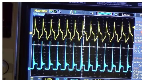
TEST with 2A impulsive current at a frequency of 100KHz
