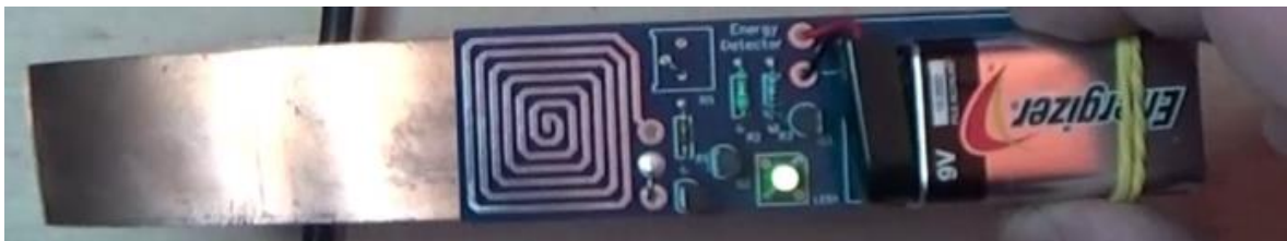
Running mode with antenna extension of copper soldered in the capacitive area on the PCB Bottom side
