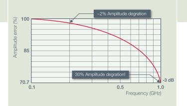
Bandwidth is defined as the frequency at which a sine-wave input signal is attenuated to 70.7% of its true amplitude (the -3 dB or 'half-power' point, shown here for a 1 GHz scope).
