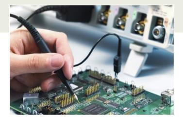
**Probing for answers:** Do you plan to measure voltage, current or both? What frequency is your signal? How large is the amplitude? Does the DUT have low or high source impedance? Do you need to measure the signal differentially? What you want to do determines the probes you need.
